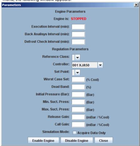
The C.R.O. to better manage the availability of the refrigeration power, it modifies the set-point of the normal temperature compressor rack controller. Execution interval set when the new set-point will be applied to the compressor rack. Back analysis interval set how far in the past the analysis must retrieve its data. Defrost
