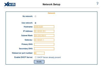
**NETWORK MASK:** is just like a filter, 255.255.255.0 means XWEB can directly reaches only PCs belonging to its own IP range. All other requests will be sent to a valid gateway.
