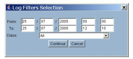
It is possible to filter all the command sent using "From", "To" and Class.
